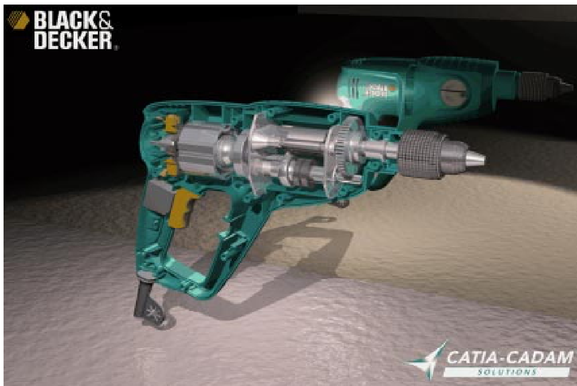
Fig. 4.28 Shaded image of a CAD geometric model ((Image appears with the permission of IBM World Trade Corporation/Dassault Systems - Model generated using CATIA))
