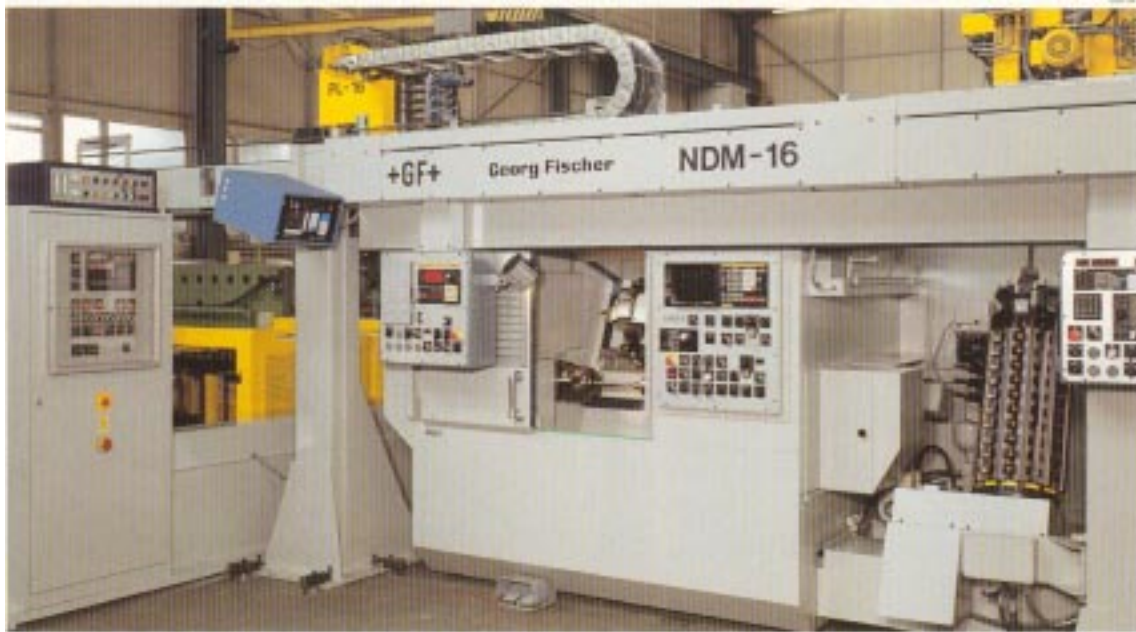
Fig. 11.23 Drum type tool magazine used in CNC turning centres with modular tooling for storing large number of tools (Courtesy Georg Fischer, Switzerland).
