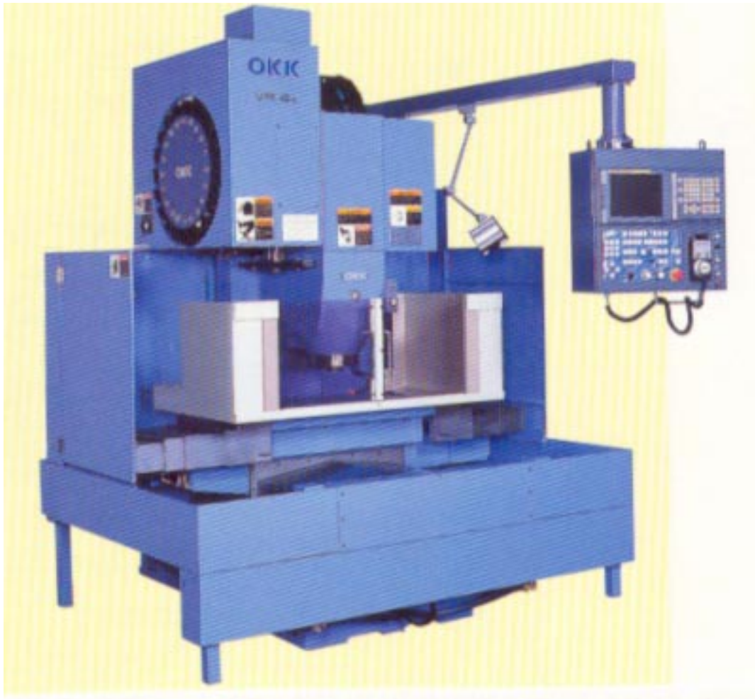
Fig. 11.16 A CNC machining centre with a drum type tool magazine (Courtesy OKK Machine tools, Japan).
