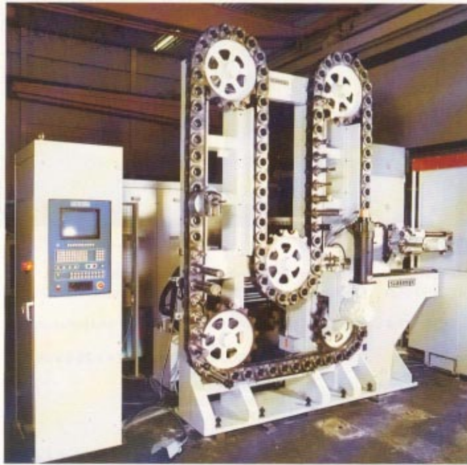
Fig. 11.19 An example of a chain type tool magazine with a capacity of 100 tools (Courtesy Dixi, Switzerland).
