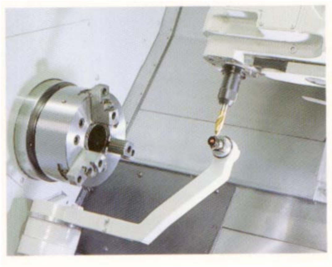
Fig. 11.13 Typical tool setter integrated with a CNC turning centre (Courtesy Yamazaki, Japan).
